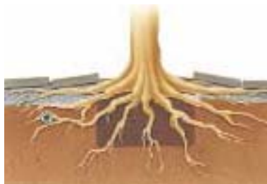
As the tree grows the roots undergo secondary thickening which begins to lift paving and cause extensive damage. Cutting roots to repair paving or excavating the service pipe will seriously destabilise the tree, probably leading to its death and removal.
