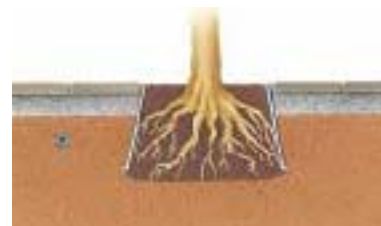
As the tree establishes, the roots spread out and are guided downwards and outwards by the root director walls and integral ribs.
