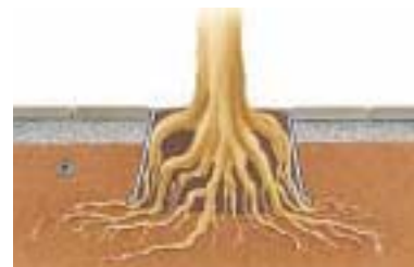
The established tree roots spread below the barrier where secondary thickening does not harm paving. Deeper root growth also improves tree stability and drought resistance.
